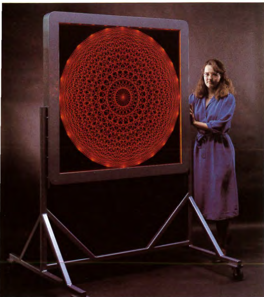
2048 x 2048 pixels 1.5 meters diagonal (59 inches) World's Largest Fully-Populated, Dot Matrix Display
